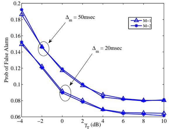
Fig. 4. Prob of false alarm for the shared cooperative spectrum sensing approach as a function of the mean time between transmission  $\Delta_m$ , for  $d_m = 5$ ,  $T_w = 0.7\text{msec}$ ,  $\tau_m = 10\mu\text{sec}$ ,  $B_w = 50\text{MHz}$ , and  $\gamma_S = 0\text{dB}$
