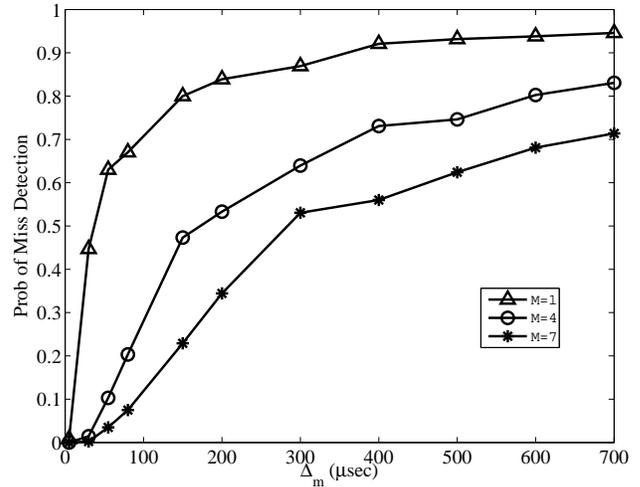
Fig. 2. Prob of miss detection for shared cooperative spectrum sensing approach wrt the mean time between transmission  $\Delta_m$ , with  $d_m = 5$ ,  $T_w = 0.7$ msec,  $\tau_m = 5$  $\mu$ sec,  $\gamma_S = 10$ dB,  $B_w = 50$ MHz, and  $\gamma_T = 10$ dB
