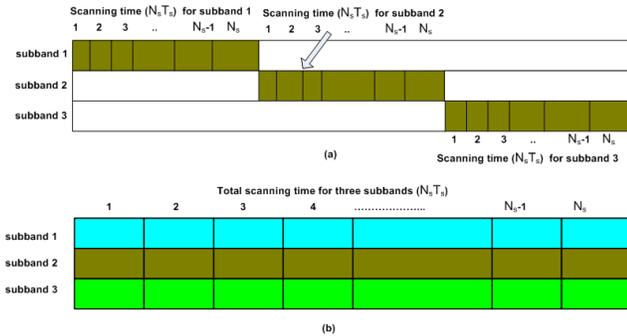
Fig. 1. (a) Cooperative scanning with  $M = 3$ : The time required to scan the spectrum (subband) is  $N_S T_S$   $\mu$ sec, (b) Non-cooperative scanning: The time required to scan is  $M N_S T_S$   $\mu$ sec, using one node
