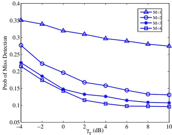
Fig. 3. Prob of miss detection for the shared cooperative spectrum sensing approach as a function of the transmission SNR  $\gamma_T$ , for  $d_m = 5$ ,  $\Delta_m = 40\mu\text{sec}$ ,  $T_w = 0.7\text{msec}$ ,  $\tau_m = 10\mu\text{sec}$ ,  $B_w = 50\text{MHz}$ , and  $\gamma_S = 5\text{dB}$
