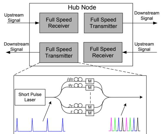
Figure 4. Hub node architecture.
