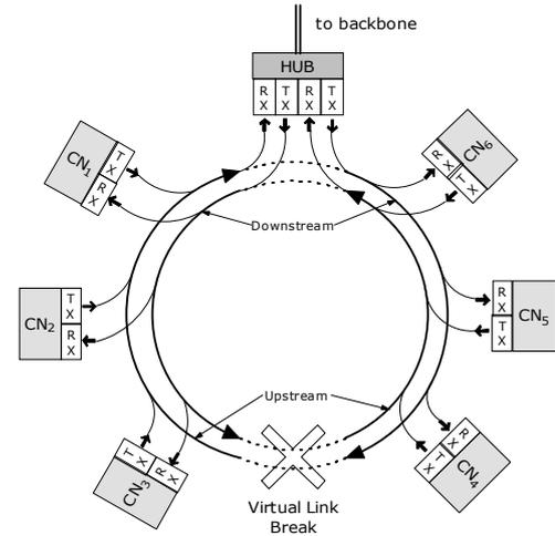
Figure 2. Traffic aggregation core network architecture.
