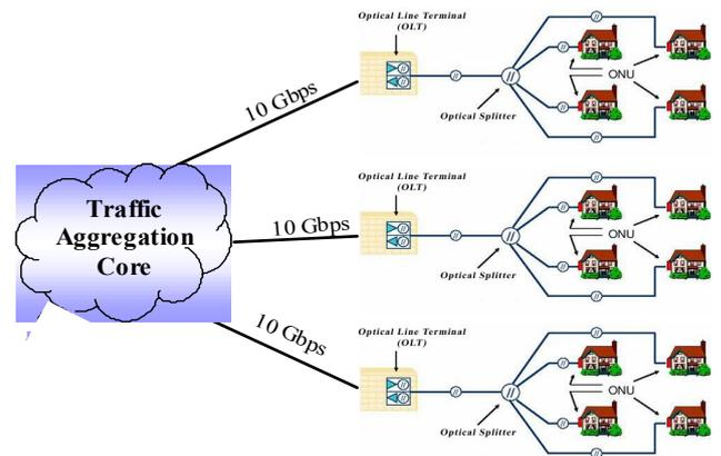
Figure 1. Example of traffic aggregation from several Passive Optical Networks (PONs).
