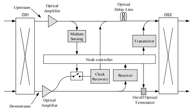
Figure 3. Client node low-cost architecture.
