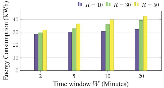
Figure 5. Impact of  $W$  on performance of DIM for different values of  $R$ . 38% while for the latter the increase is *only* 17%. Two are the main reasons: i) the LEDs used in DIM are more efficient than HPS lamps used for DEL, ii) the DIM checks presence of nearby users every more often than DEL.
