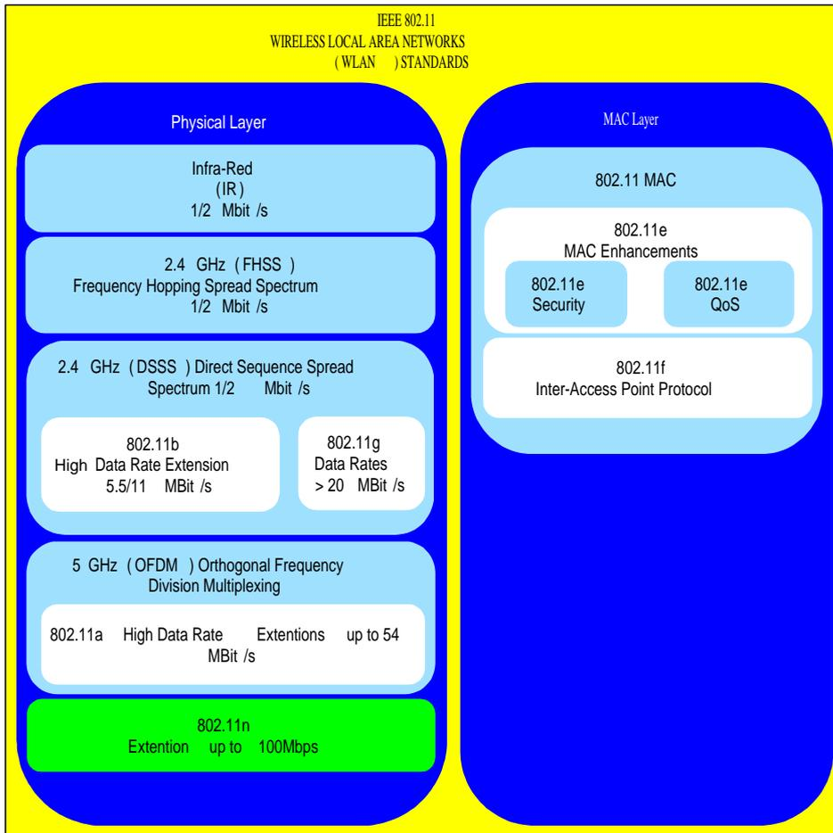
FIG. 2.3. IEEE Wireless Local Area Network (WLAN) standards.
