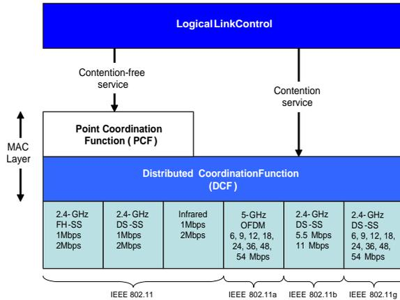
FIG. 2.1. Overview of the IEEE 802.11 Protocol Stack.
