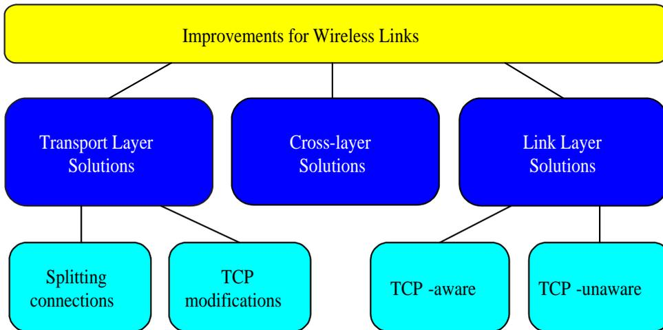
FIG. 4.1. Graphical classification of possible improvements for 802.11 wireless networks.
