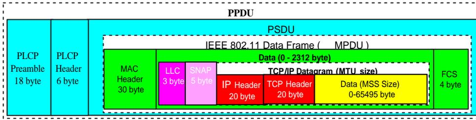
FIG. 3.1. Packet encapsulation in TCP over 802.11 networks.[11]
