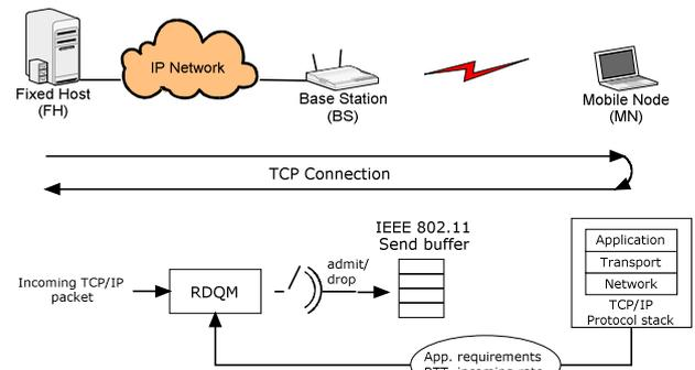
Figure 1. Receiver-Driven Queue Management (RDQM) architecture.
