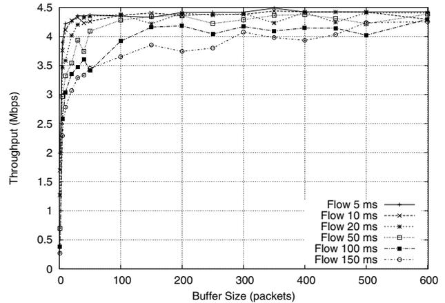
Figure 4. Single-flow throughput as a function of buffer size.
