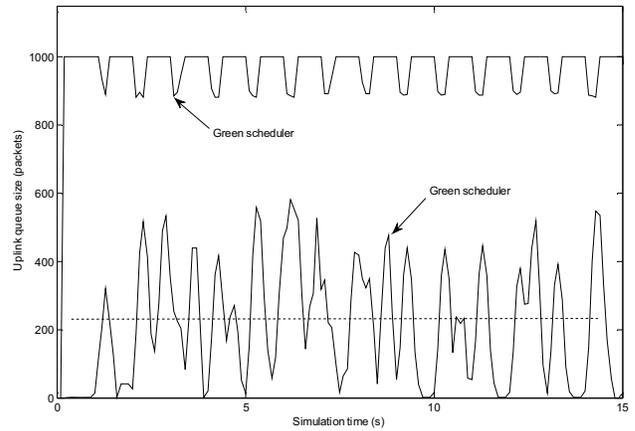
Figure 8. ToR switch uplink buffer occupancy.
